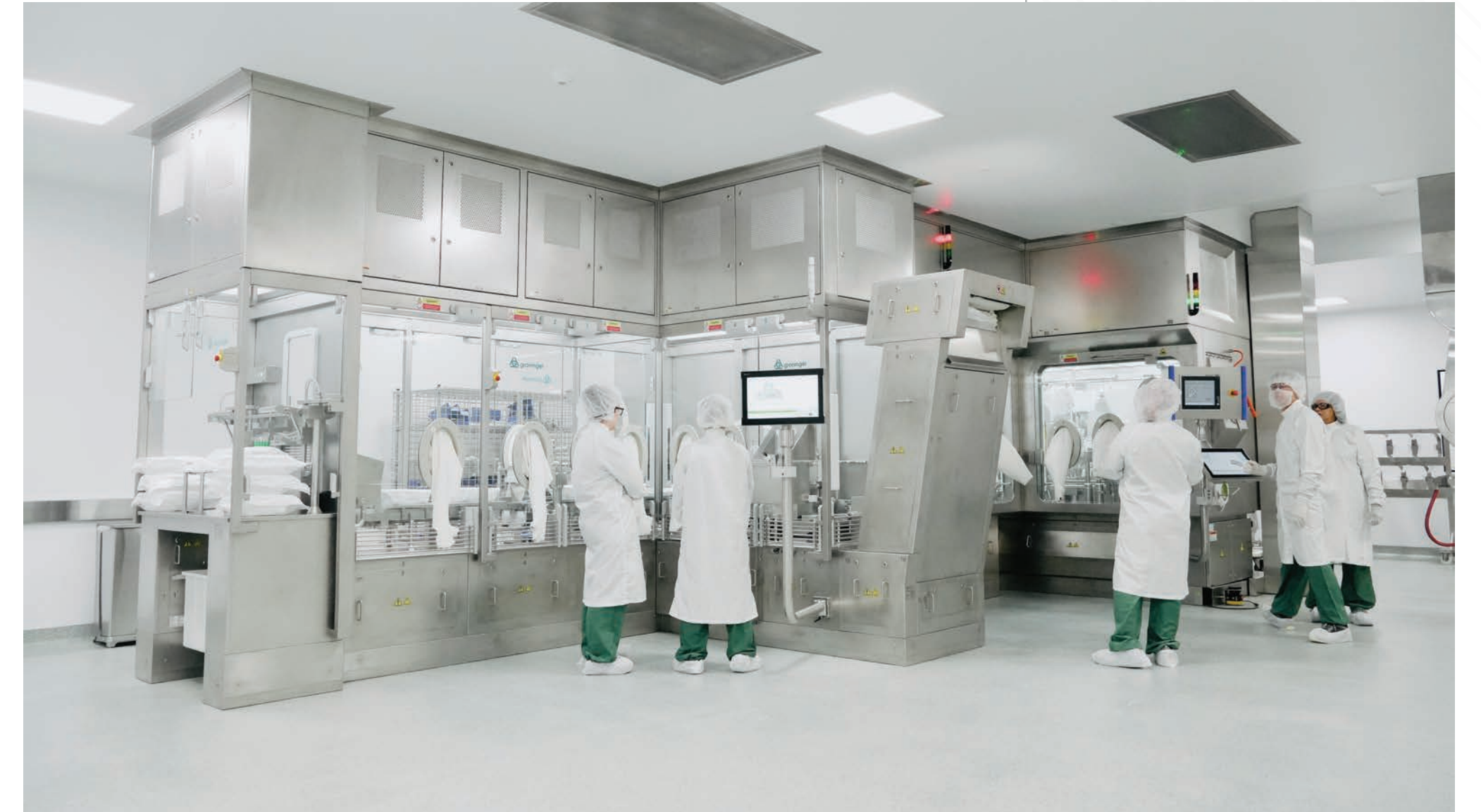
Groninger nest filling line with SKAN isolator2
