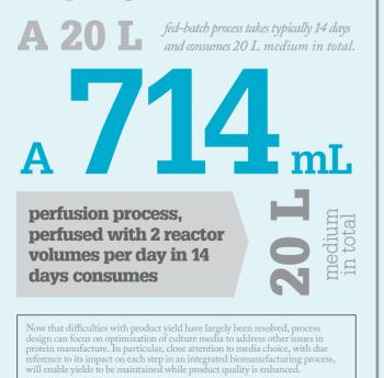
A modern process: In a bioreactor with a volume of:
