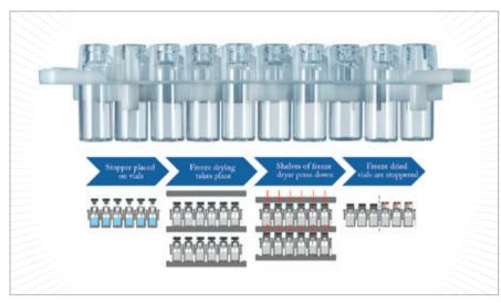
Figure 1. Freeze drying process.
