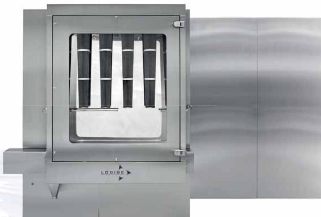
Lödige has rounded off its product portfolio for continuous granulation with a new dryer: the LCF 5 is distinguished by a defined retention time of the product inside the machine. This enables shorter processing times to be achieved in production. With the LCF 5, CoriMix® CM 5 laboratory ringlayer mixer and customized dosing technology, Lödige now offers a complete continuous GRANUCON granulation line.
