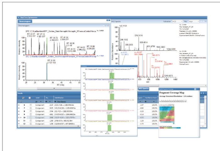
Figure 4. Peptide Mapping analysis of Trastuzumab. Main process & review page in BioPharma Finder software with interactive plots and tables for user friendly data mining.
